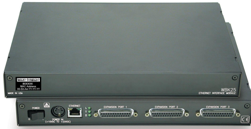
The WBK25 Ethernet-to-Parallel Port Interface
