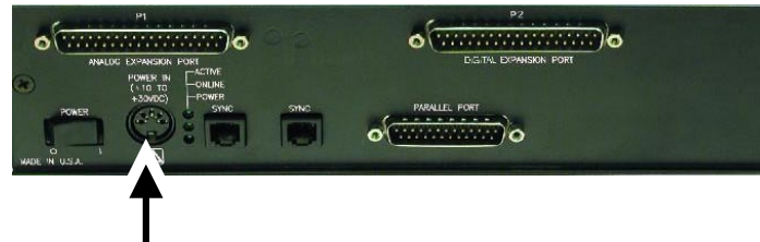
DIN5 POWER IN Connector (+10 to +30 VDC)
